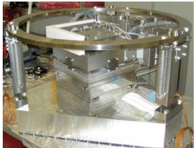
The high-precision stage in IMS's eMET proof-of-concept system as delivered by Philips Innovation Services.
