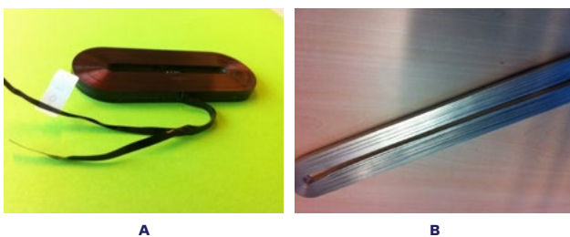
Figure 9: Copper (A) and aluminum (B) foil coils
